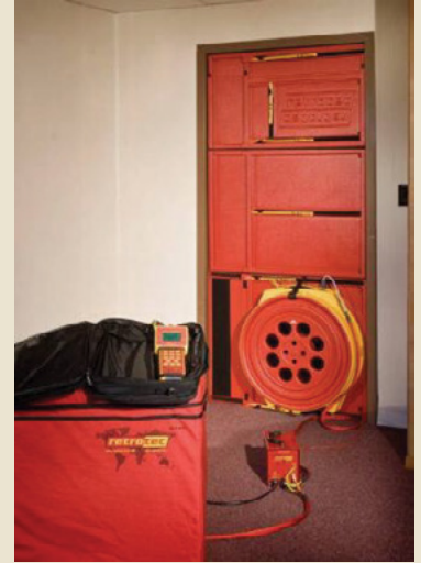
Figure 5.2 Fan-door equipment setup (photo courtesy of Retrotec Energy Innovations Inc., Vancouver, B.C.)
