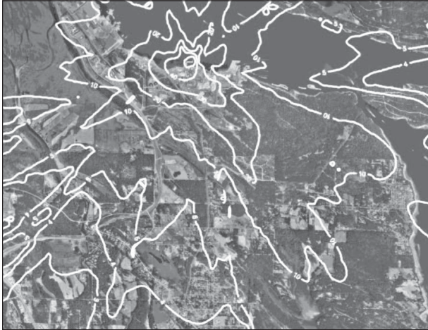
This figure shows the dispersion of an airborne contaminant (white contours) from the emissions stack of a proposed powerplant for a coastal BC town. The proposed power plant is located at the centre of the smallest contour. The dispersion contours were produced with a computer model. Image used courtesy of BC Hydro.
